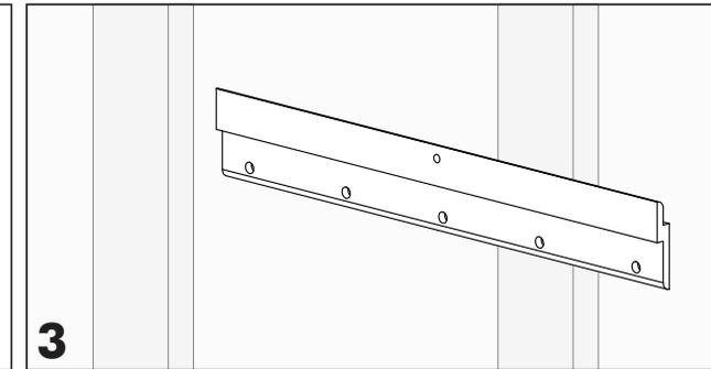
Secure the second included bracket to the wall. We recommend securing this bracket into at least one stud in conjunction with another attachment method. If the chosen location does not allow stud attachment, we recommend using toggle bolts. Your unique installation requirements may require an alternative solution.
