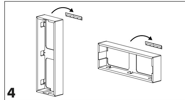
Hang the On-Wall Frame on the wall mounted bracket by aligning the (2) brackets. Please Note: The bracket attached to the On-Wall Frame will need to be lifted slightly above the bracket on the wall so it can drop down into the bracket affixed to the wall surface.
