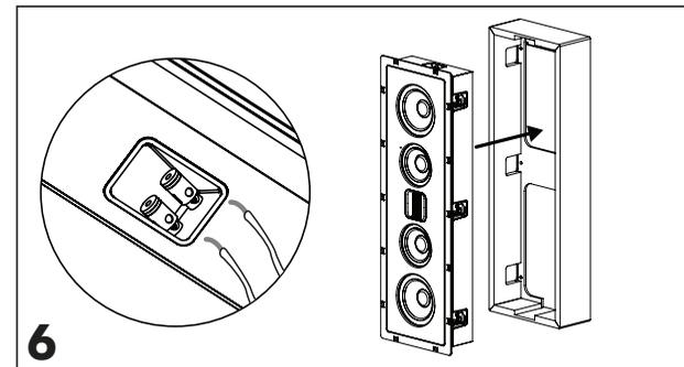
Pull the wires designated for the speaker through the On-Wall Frame and attach them to the binding posts of the speaker. Be careful to maintain proper polarity (Red (+) to Red, Black (-) to Black). Then place the speaker in the frame. Tightening all the mounting locks securing the speaker into the frame.
