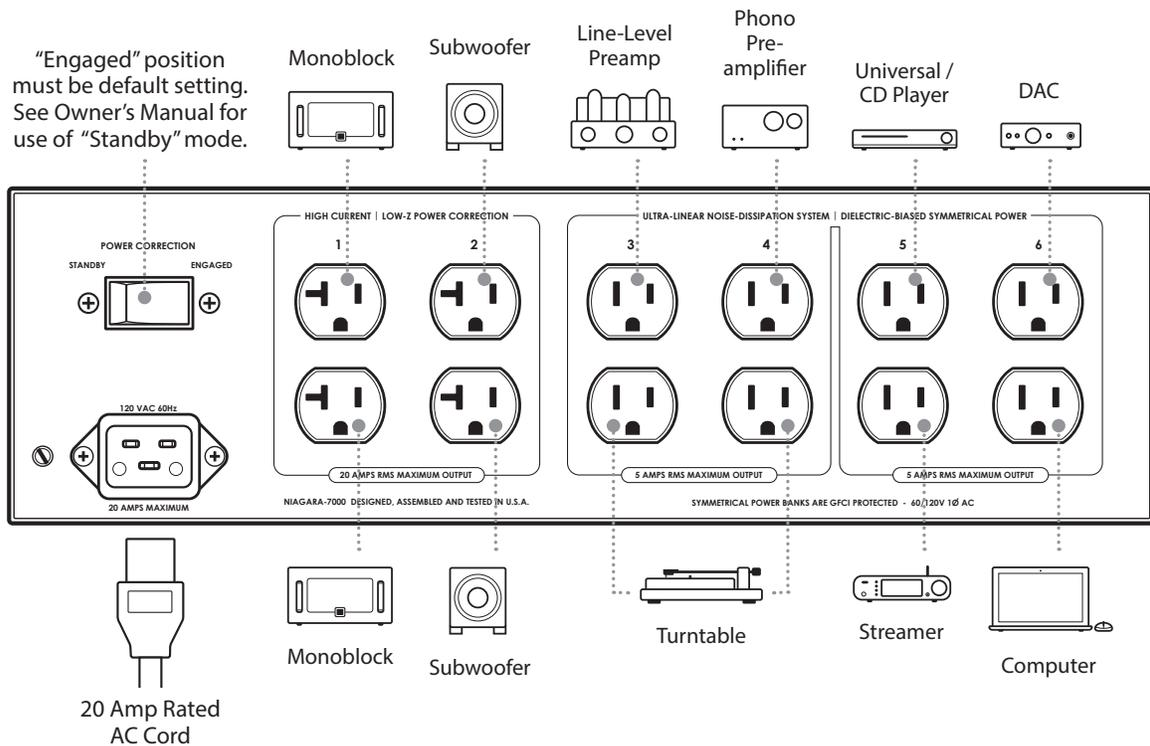
**Note:** Banks 3 through 6 are subject to many variables and circuit conditions, so experimentation for best results is encouraged. Power amplifiers **must** be connected to Banks 1 or 2.
