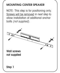
Position bracket and ensure it is level. Mark the two <u>center</u> screw holes. Drill pilot holes, then press anchor bolts firmly into drywall and screw in. Follow with flathead screws: DO NOT SCREW ALL THE WAY IN AT THIS POINT—leave screw heads protruding slightly.
