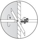
**WARNING!** All screws must be inserted straight and fully tightened to ensure correct operation of anchor bolts.
