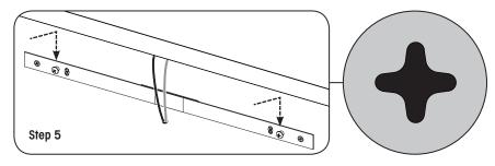
Align keyhole slots (see inset) on rear of speaker with protruding screw heads on the bracket, then using an "in and down" motion mount speaker on bracket.
