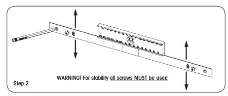
Bracket is slotted *(see illustration)*, to allow further adjustment if necessary. Re-check to ensure bracket is level. Mark <u>outer</u> screw holes.
