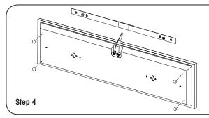
**NOTE:** When wall-mounting the **Millenia LP 2**, attach the 4 self-adhesive bumper pads to the back of the speaker.
