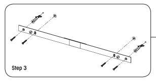
Remove the two flathead screws (not shown). Drill inner pilot holes then press anchor bolts firmly into drywall and screw in. Now insert all four flathead screws and tighten.
