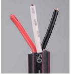
Strip the dielectrics leaving some of the red PVC exposed. Strip the black and white PVC as close to the jacket as possible and tightly twist them together. Trim off the excess conductors.
