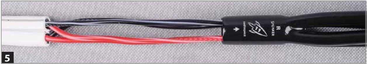
5. Feed the leads into the pants carefully so that the correct lead is in the correct leg of the pants.
