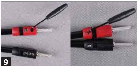
9. Insert the Red wire pair into a red-stripe speaker connector and tighten the connector's screws using a hex allen wrench. Insert the Black wire pair into a black-stripe speaker connector and tighten the connector's screws using a hex allen wrench.
