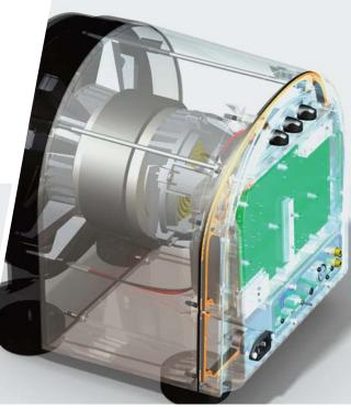
The fully integrated heat-dissipating Ultra-Class  $D^{\mathsf{TM}}$  amplifier follows the shape of the cabinet maintaining the overall low profile. The amplifier is mounted directly to the amplifier plate to provide both EMI and shock protection. Preamp cover eliminates any possibility of air leaks.
