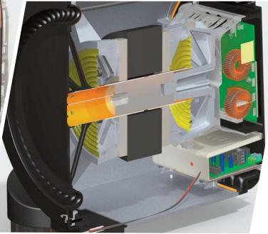
**Ultra-low distortion split voice-coil design** with an extremely long winding width allows for an incredible two inches of linear excursion with vanishing low levels of distortion. Shallow die-cast driver basket and two-piece flattened cone construction contribute to the compact footprint.
