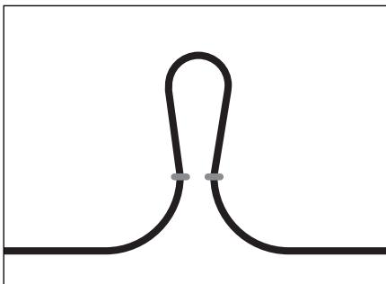
2. Recommended: Use a wire tie (not included) to keep the wire loop intact and it will act as a strain relief.
