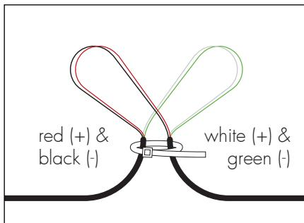
4. Cut the red (+) and black (-) **OR** white (+) and green (-) wires with cable strippers and strip off 1 inch (25.4 mm) of insulation to expose the bare wire conductor.
