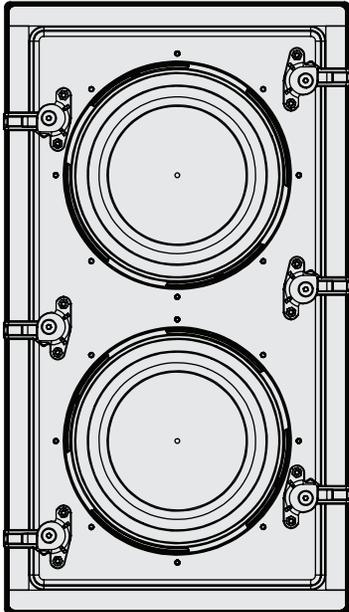
OVERALL DIMENSIONS: (H) 19.11" [486mm] x (W) 10.73" [273mm] x (D) 4.1" [103mm]
